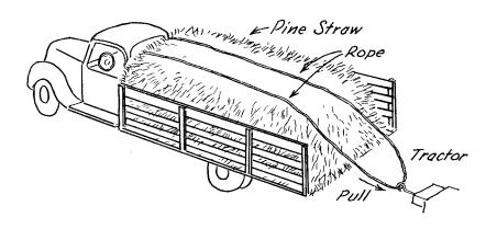
The two ends of a thirty-foot piece of one-inch rope are fastened to two stake sockets at the rear of the truck bed. The rope is laid along the bed of the truck with the two strands about four feet apart. The surplus rope is placed on the truck cab.
