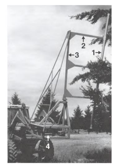
Figure 1—The 1997 lower-crown branch shaker is shown properly positioned within the perimeter of the crown. 1 = energy bar; 2 = horizontal support; 3 = vertical drive shaft; 4 = crank arm.
