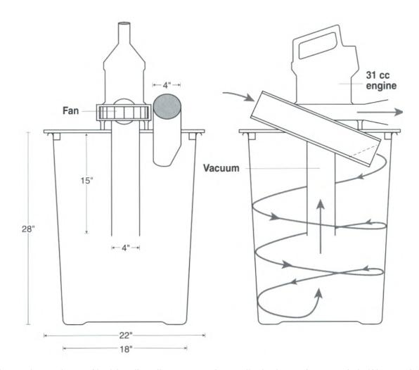
**Figure** 2—Specifications for assembly of the pollen collector, comprised principally of a plastic garbage can and a leaf blower, with the resulting air flow pattern.
