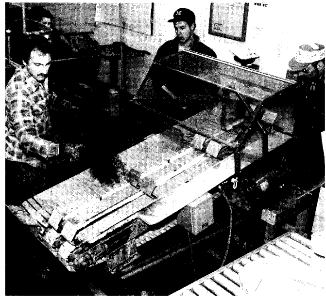
Figure 4—Prototype root pruner has been tested at the Forest Service's Coeur d'Alene Nursery.
