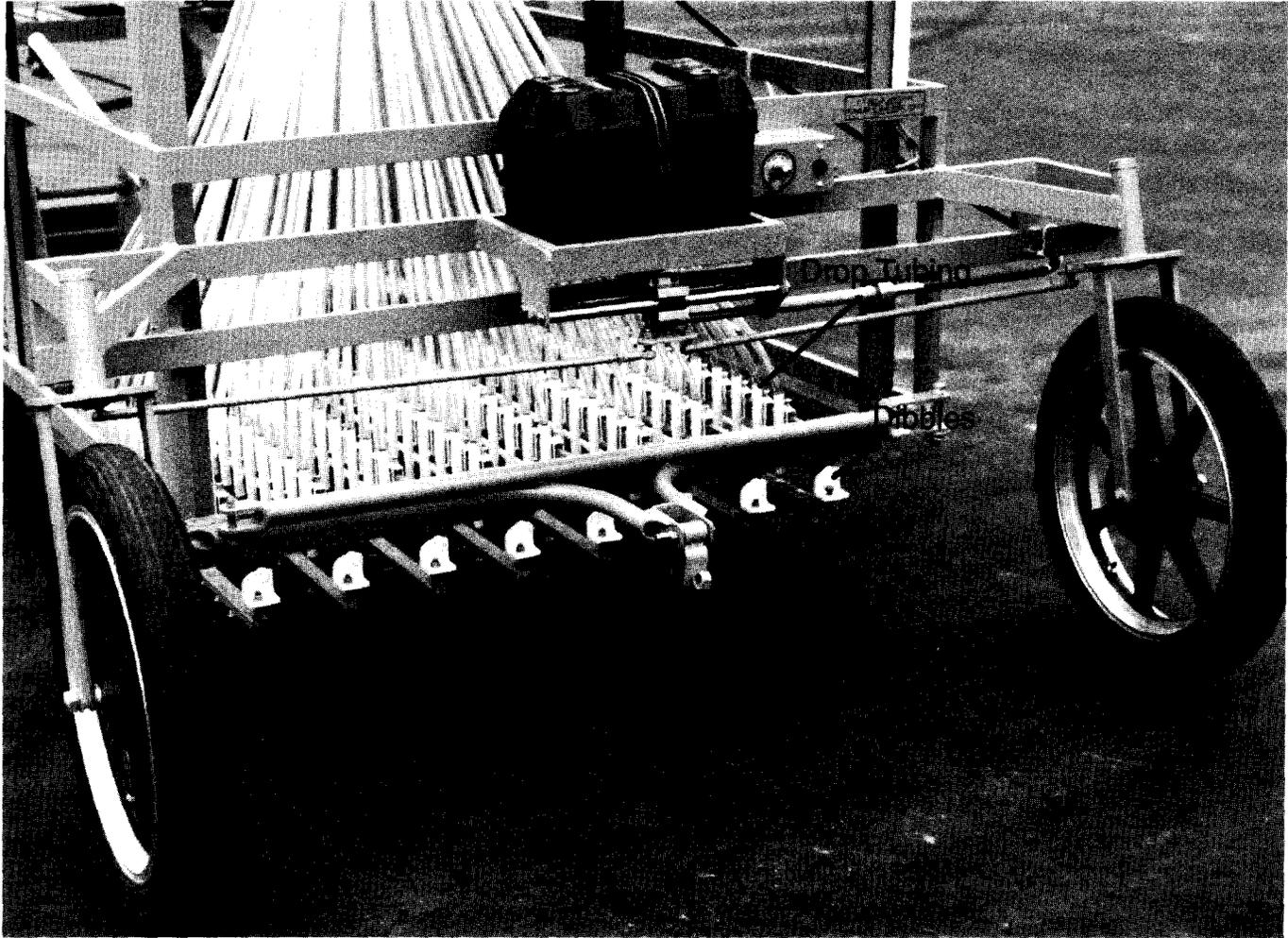
**Figure 3**—Close-up of the tubing and the dibbles.
