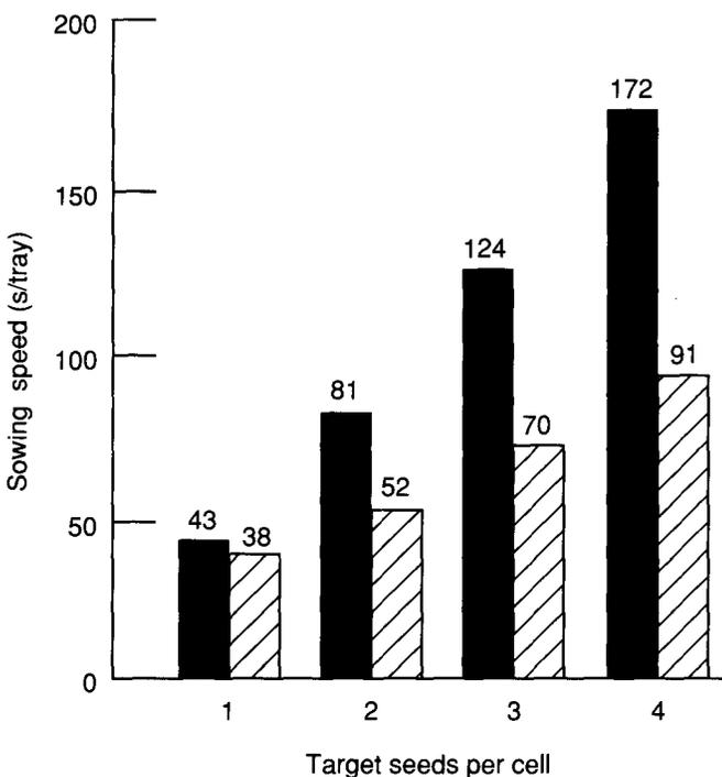
**Figure 3**—Sowing speed (s/tray) versus the target number of seed/cell for ponderosa pine (solid bars) and western larch (hatched bars) at a constant seed-supply setting of the vibrating feeder bowl (trial 2).
