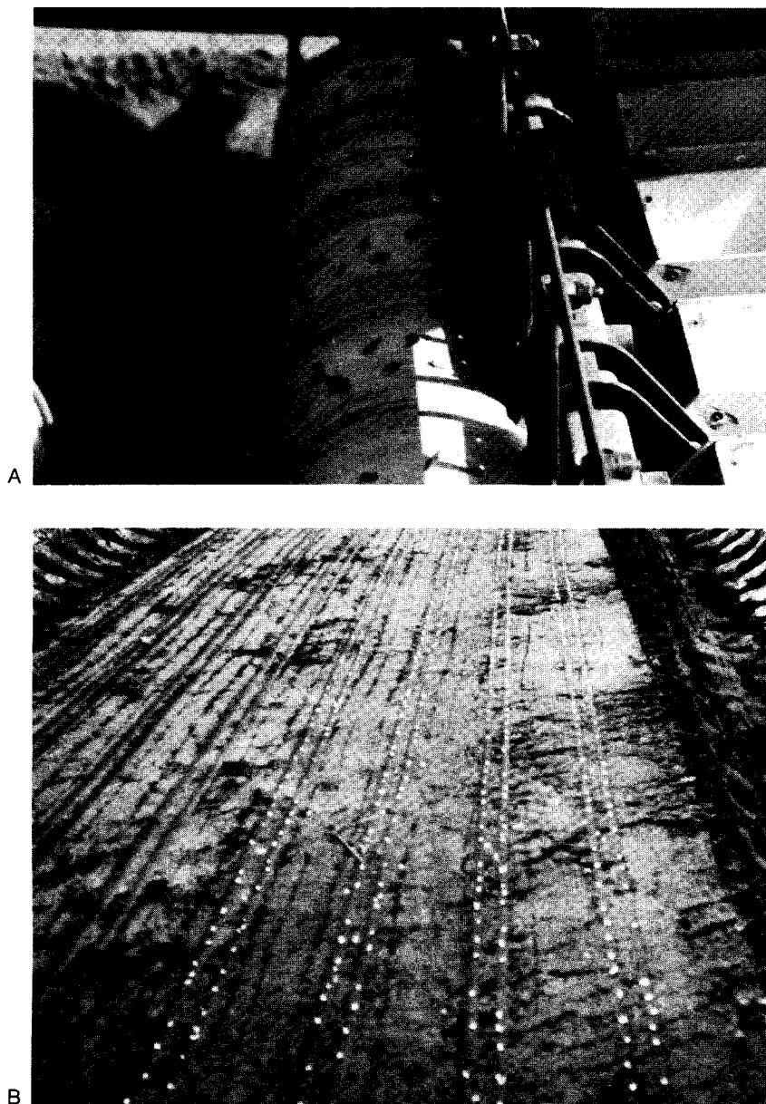
Figure 2 —Longleaf pine seeder with custom-built vacuum seed drum (A) designed for precision sowing of 8 offset double rows per seedbed (B).
