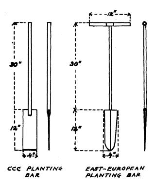
The CCC bar has a sharpened end, but the European form has sharpened sides, too; therefore, it penetrates easier into the ground, especially when the ground is unprepared and full of roots and stones. The European form weighs 5 to 6 pounds; the CCC bar, 8 pounds. The wooden horizontal handle makes the European form handier for the work, especially for physically less strong workers.
