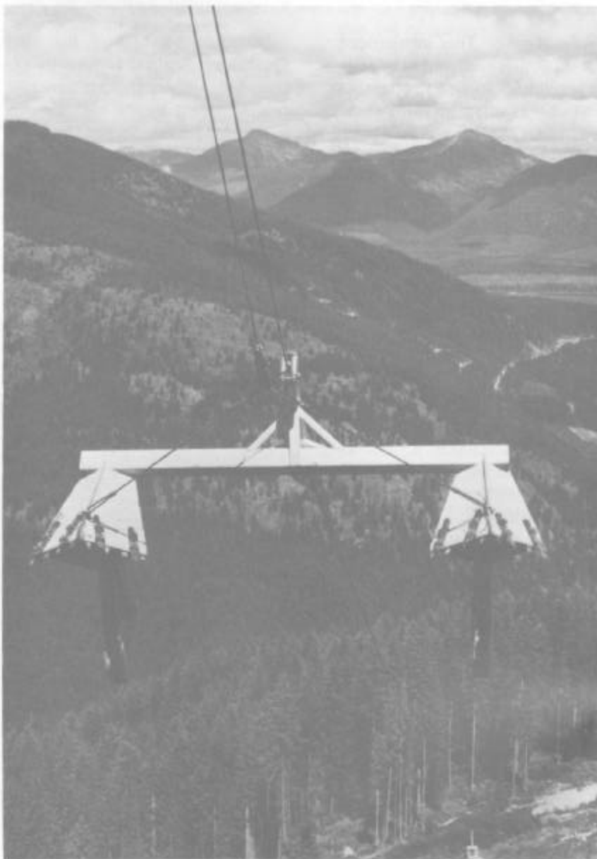
Figure 1—Scarifier implement rides skyline cable downslope to begin digging planting spots.
