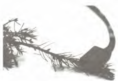
Figure 1—Douglas-fir seedling with electrode from oscilloscope/square wave apparatus attached.
