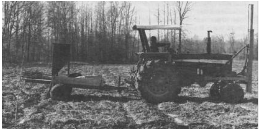
Figure 1.—Tractor-mounted hydraulic punch with sand hopper-equipped trailer carrying whips.
