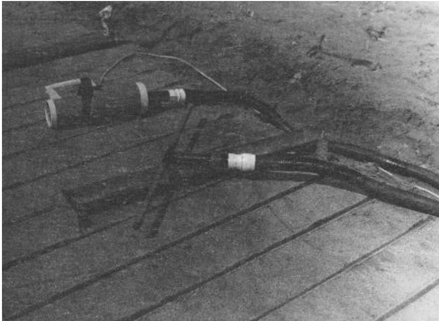
Figure 4. — A concave metal tray concentrates seeds for easy pickup by the vacuum system.
