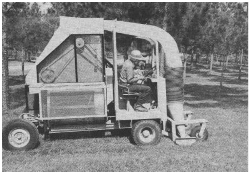
Figure 1. —The Bowie Vac-U-Seed Harvester undergoes testing at a Mississippi seed orchard.
