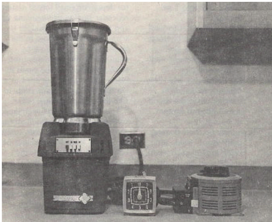
Figure 1. —Three-speed commercial blender (mixer), variable speed autotransformer (rheostat), and timer used to depulp Juniperus cones.
