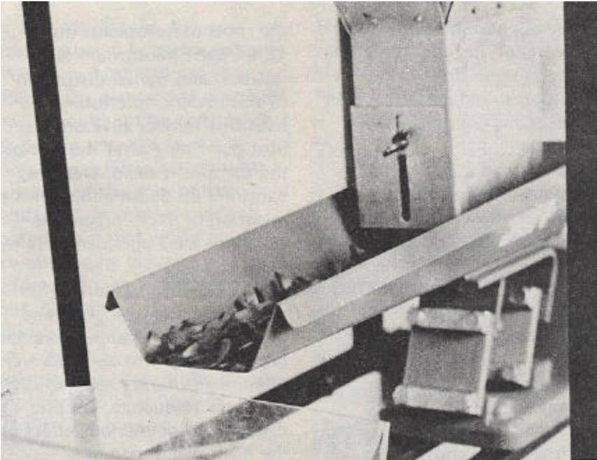
**Figure 3.**—Vibrating feeder funnels seeds into dewinging cylinder.
