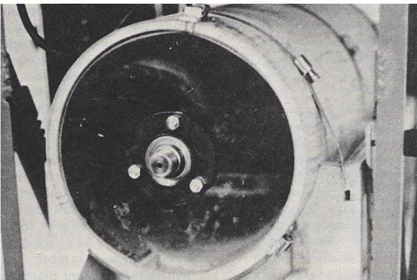
**Figure 4.**—Central shaft rotates rubber flaps, dewinging seed.
