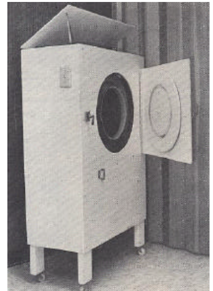
Figure 1. —The seed extractor with hatch and lid open.
