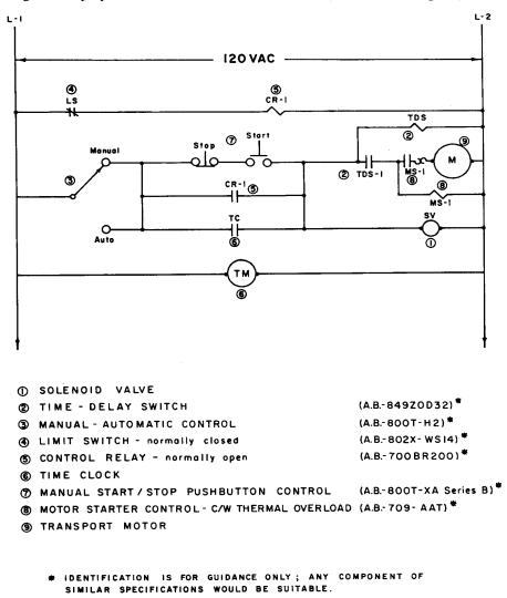
Figure 1.—Schematic control circuit for boom sprinkler.
