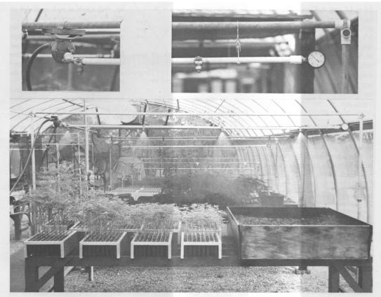
Figure 1.-An easily-built, inexpensive oscillating irrigation sprayer provides for uniform and accurate application of water and fertilizer in small nurseries.
