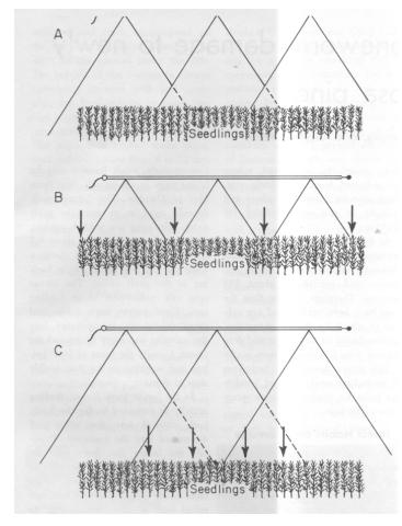
Figure 3.-Side view shows proper and improper spray patterns: (A) proper height of spray nozzles results in uniform water distribution; (B) nozzles too close to seedlings result in too little water in spray overlap areas and at edges; (C) nozzles too far above seedlings result in too much water in the spray overlap area and at edges. Arrows show areas where water distribution is not uniform.
