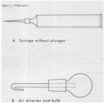
A typical pollen gun is shown in figure 1. Several workers including Crane et al (1). Serr and Forde (3) have used variations of the hypodermic needle to inject pollen into bags. Ours is an exact copy of those used in the University of Florida pine tree improvement program. Piece A is half. filled with pollen: then B is inserted into A. Squeezing the bulb forces
