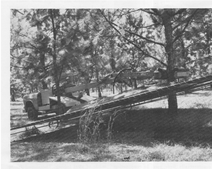
Figure 2.-Drive-into frame shown with shaker. Test Results
