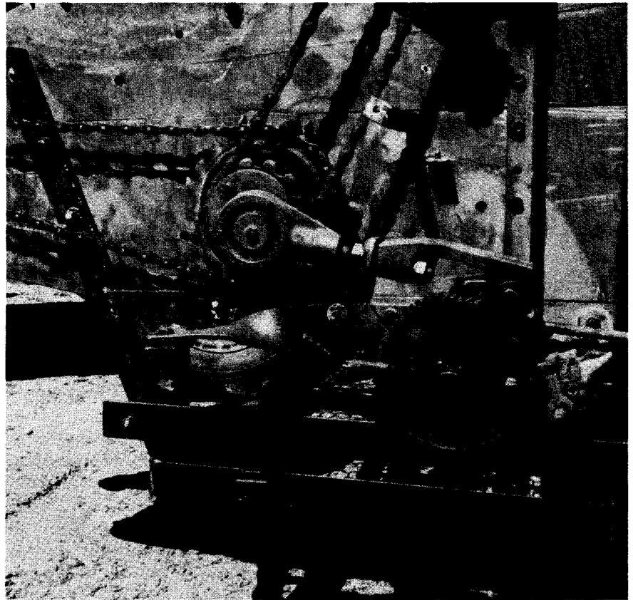
Figure 1.—Sawdust shaker drive assembly attached to the manure spreader's drive mechanism.
