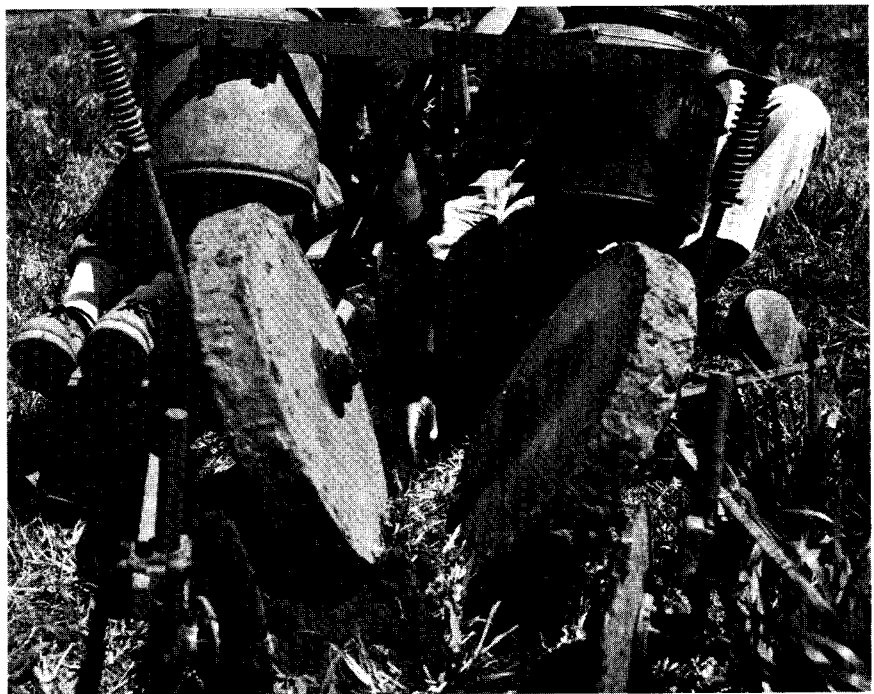
Figure 1.—This tree planting machine with a subsoiler trencher and two packing wheels opened a trench too shallow for most nursery stock and does not pack the soil uniformly about the roots.
