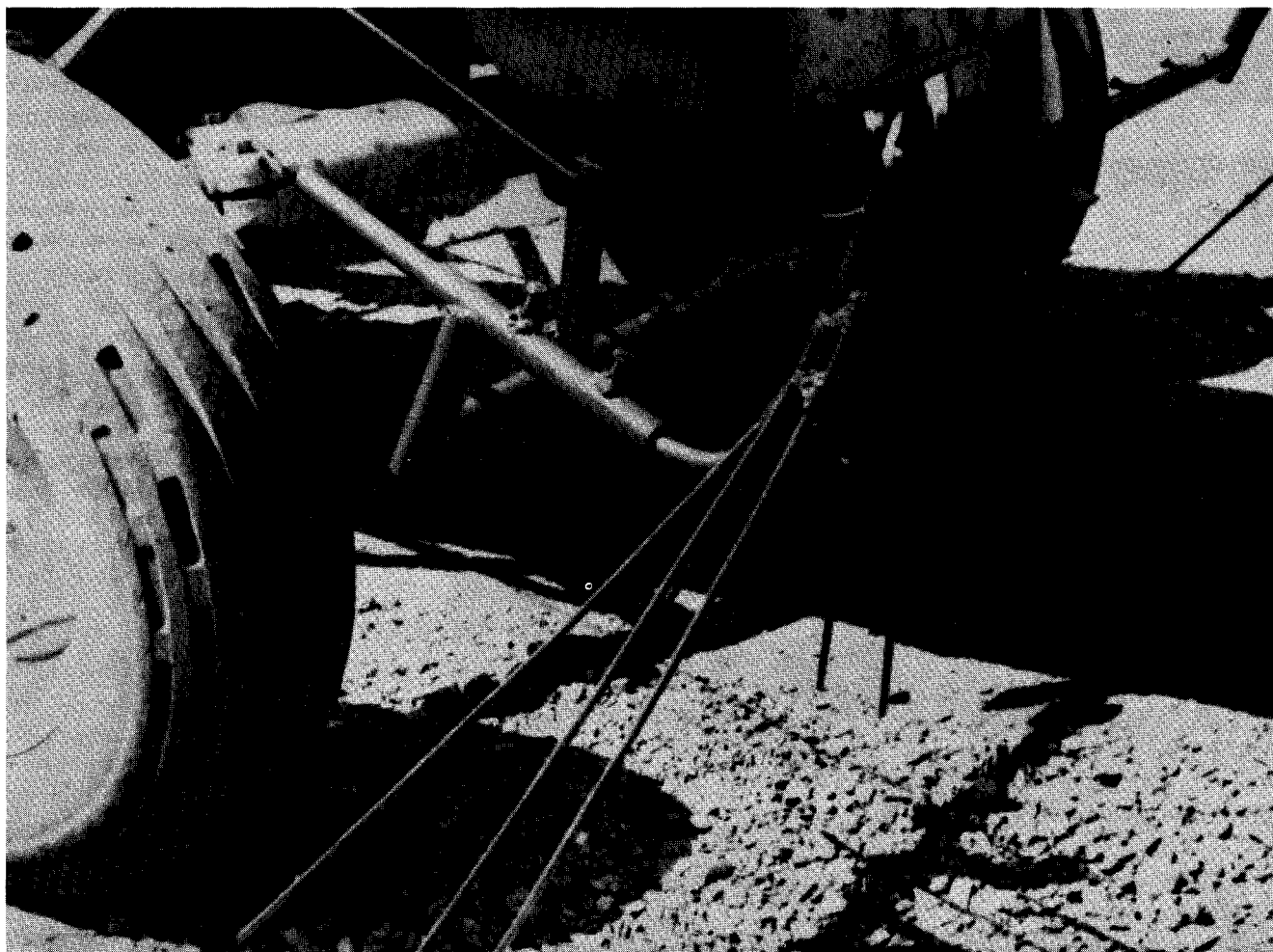
Figure 1.—A closeup of front row separator which the tractor operator adjusts with the rod attached to the angle iron.
