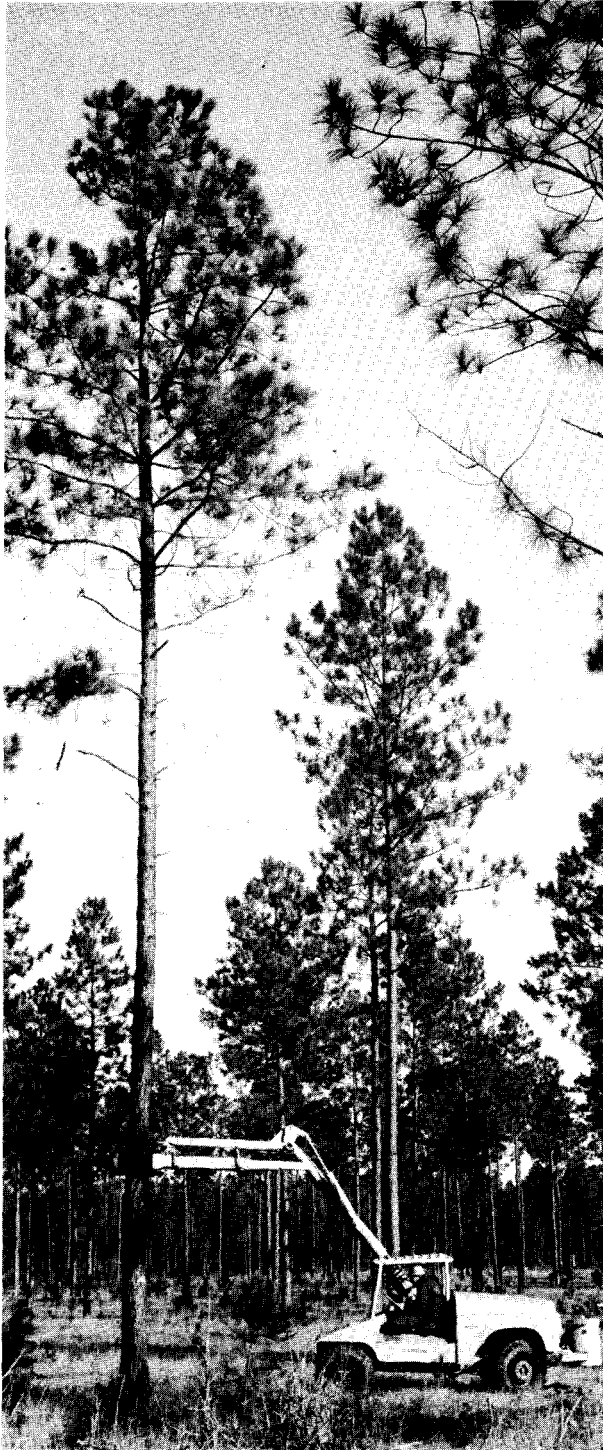
Figure 1.—Side view showing tree shaker position for shaking the tree.
