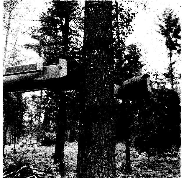
Figure 2.—View showing the padded clamping device in the open position.
