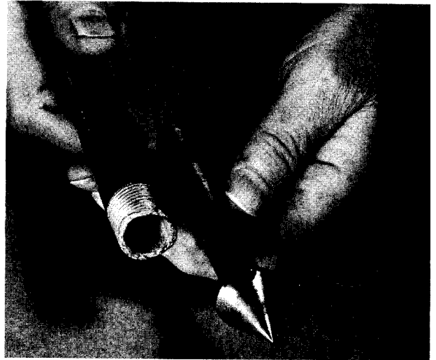
Figure 1.-The shank of a hardened steel point is inserted in the pipe, which is then driven into the soil. Once at the desired depth, a steel rod is inserted in the pipe to drive the shank of the point out of the pipe, leaving the end unobstructed.
