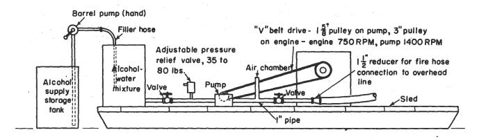
INJECTION PUMPING SYSTEM FOR APPLICATION OF ALLYL ALCOHOL
