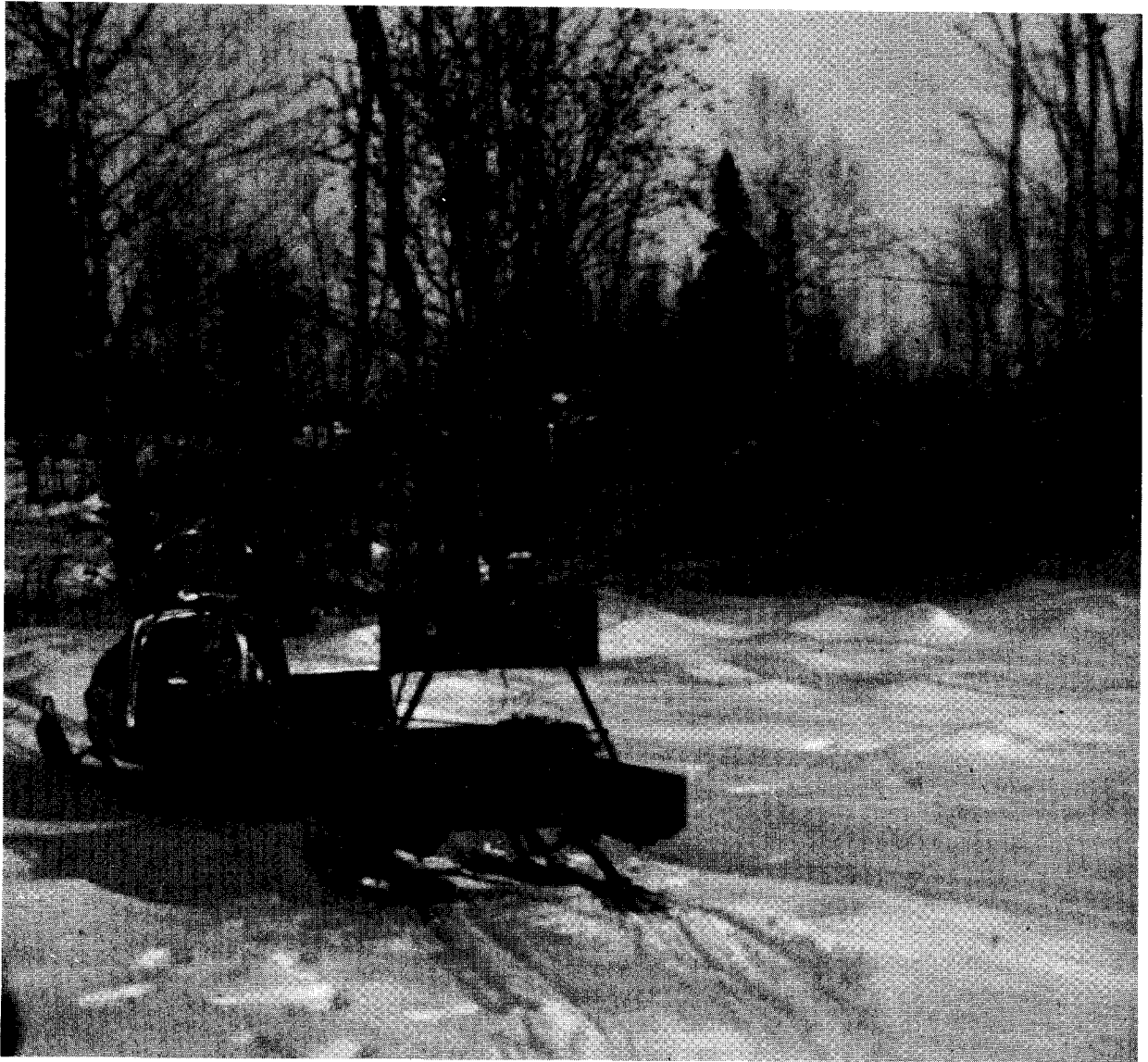
Figure 1.—View of automatic broadcast seeder mounted on sled pulled by snowmobile. Later improvements now have seeder mounted directly on snowmobile, thereby eliminating the sled and speeding up the operation.
