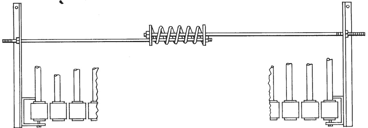
Figure 4.--Schematic diagram of unit for applying pressure to belts to prevent plants from being pulled from belts during harvesting.
