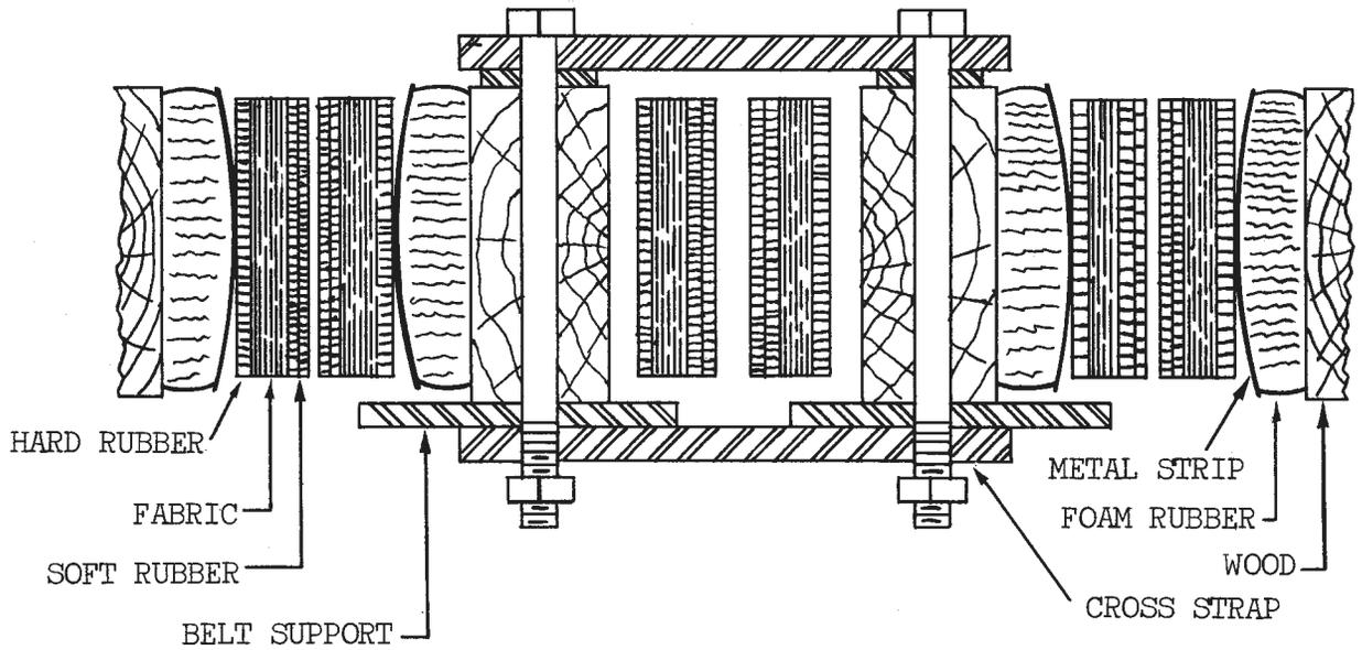
Figure 5.--Typical cross section of one lifting belt unit from the Georgia seedling harvester, showing construction details.
