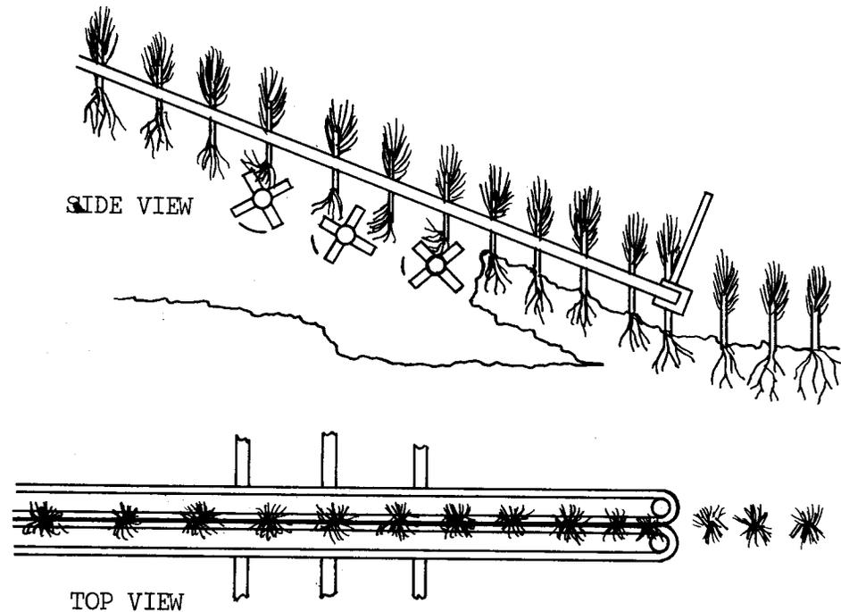
Figure 2.--Schematic drawing of lifting belts and soil removal agitators used in lifting forest tree seedlings with the Georgia seedling harvester.
