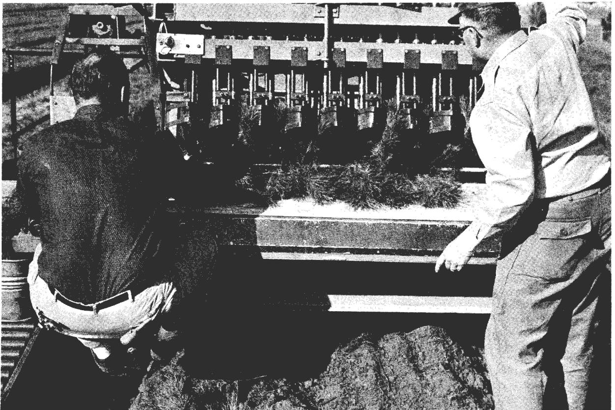
Figure 6.--Rear view of Georgia seedling harvester showing plants being discharged from lifting belts, trip bar, and cross conveyor system.
