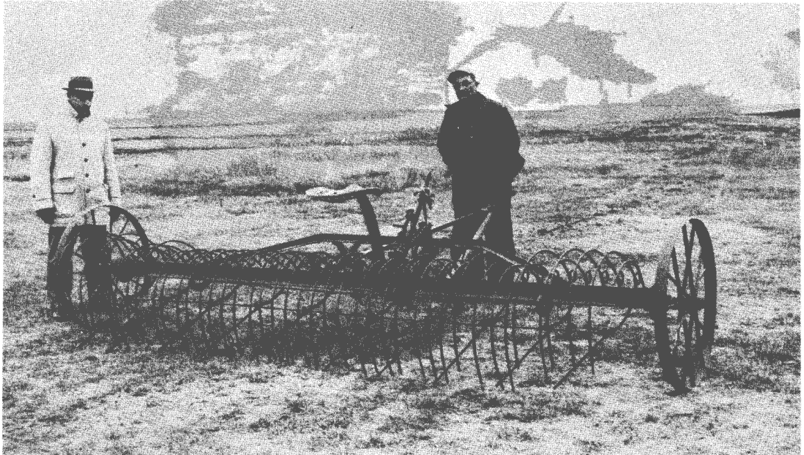
Figure 1.--Hay-rake tree cultivator.--This outfit is used to cultivate young trees by the over-the-row method. Note that sulky plow wheels have replaced the regular wheels. Oswald Pfeiffer (right), farmer at Fessenden, developed this outfit. Shown with him is Orville Overboe, SCS.
