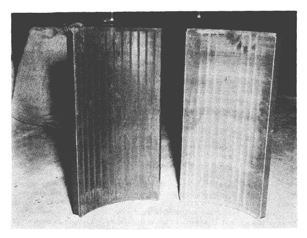
Figure 2. - <u>Right</u>, Corrugated rubber liner from Crippen Model EP polisher worn smooth by abrasive action of seed. <u>Left</u>, New liner; corrugations are 1/8 inch deep.
