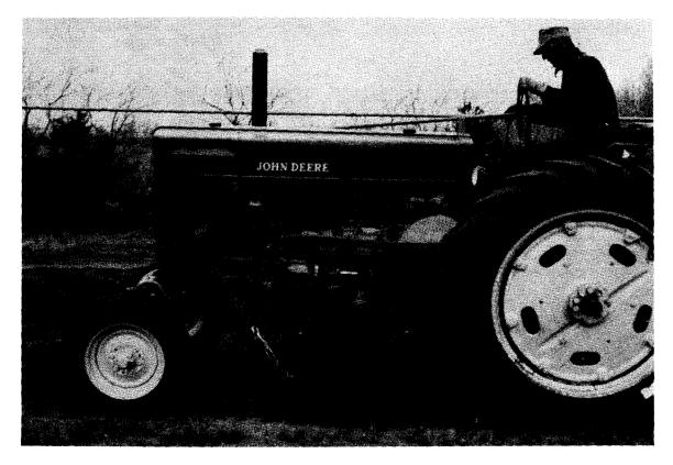
Figure 1. This tractor-mounted tree lifter was designed to undercut, side prune, and lift experimental aspen seedlings.
