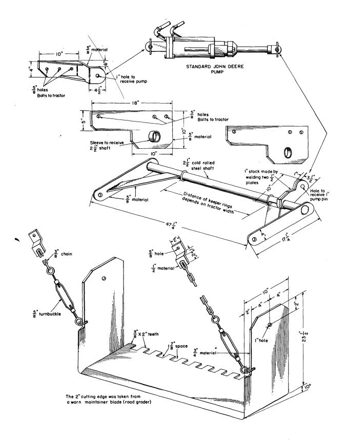
Figure 4. - Construction details of lifter.
