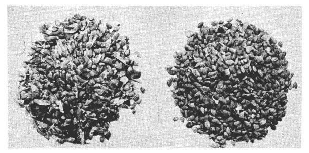
Figure 1. - <u>Left</u>, Seed improperly dewinged by Crippen Model EP polisher because of worn corrugated rubber liner. <u>Right</u>, Seed properly dewinged after liner was replaced.
