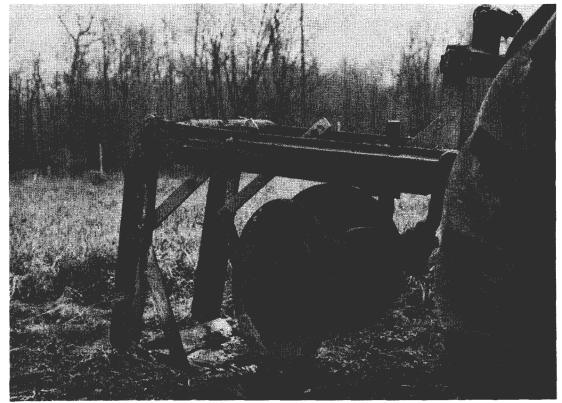
Figure 1. - Lifter in action. Chain hook up and turnbuckle determine angle of blade at a certain depth. The 1-inch bolt holding blade to hanger has a double nut to allow blade to swing.
