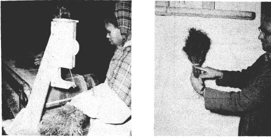
Figure 1.- <u>Left</u>, Tape dispenser ready for next bundle. <u>Right</u>, Taped bundle ready for packing.
