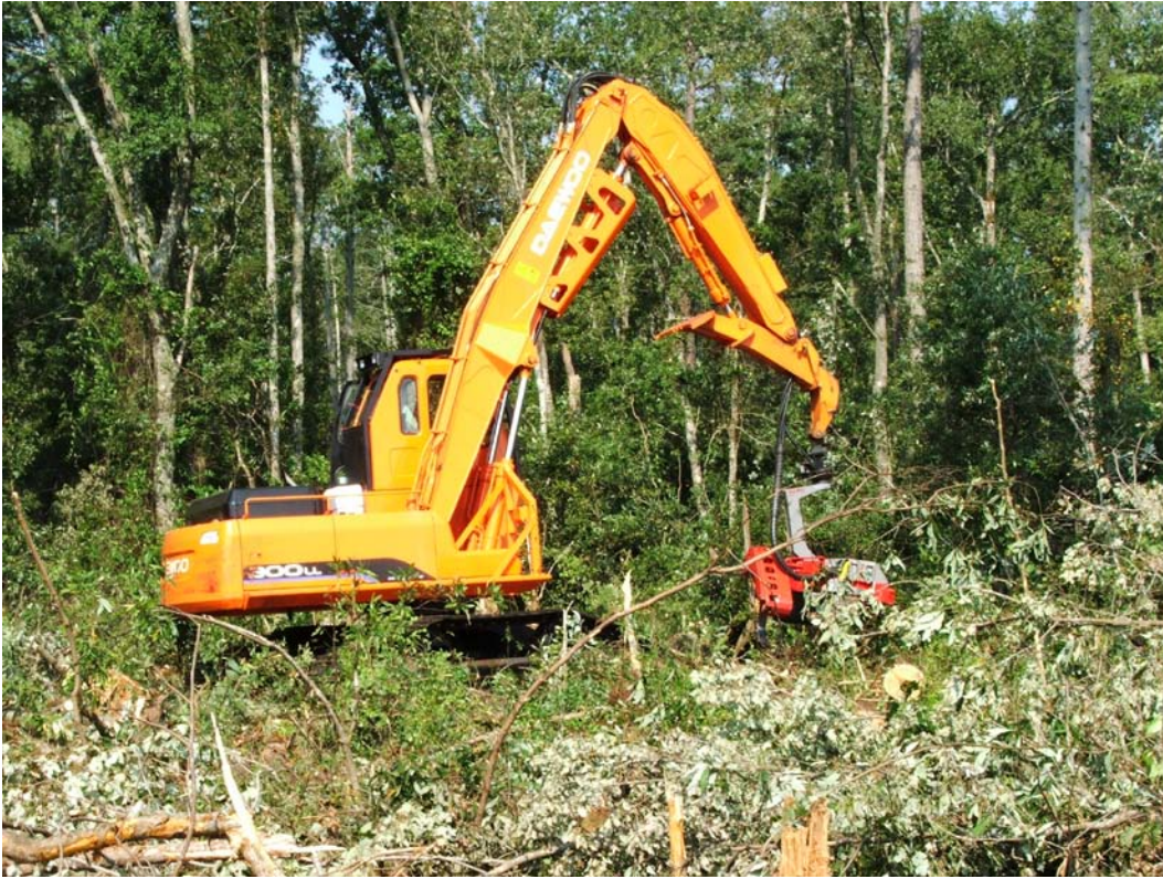
Figure 5 - Daewoo excavator with processing head.
