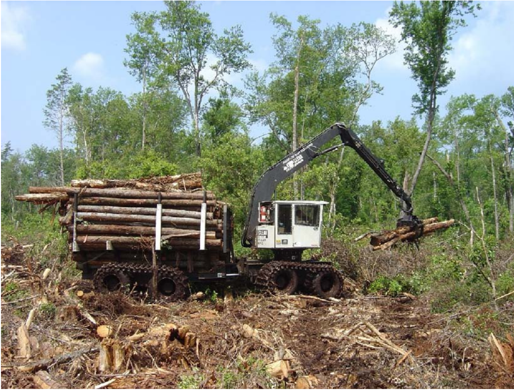
Figure 6 - Tracked forwarder collecting processed cedar logs
