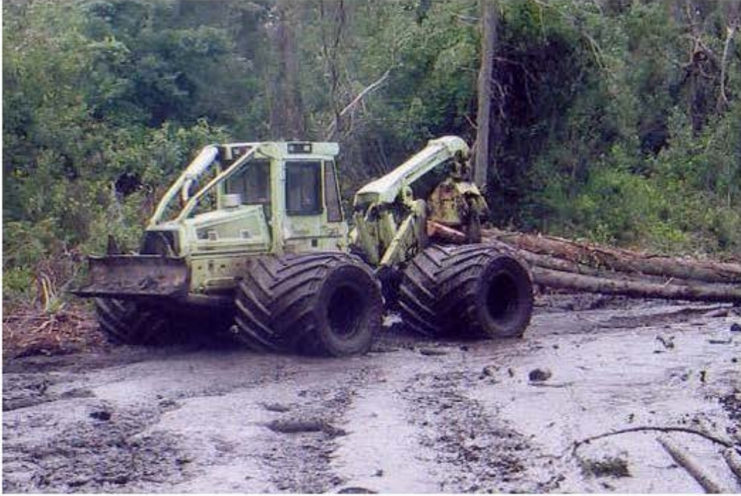
Figure 3—Hydraulic Grapple skidder used to salvage log the Blackwater Cut, courtesy of Brian Martin
