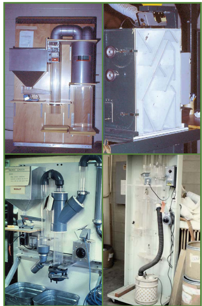
Figure 52 Various configurations of aspirators used for final cleaning.
