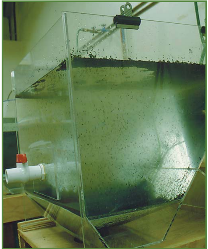
Figure 55 Separation of debris and empty seeds through the soaking of stratified seeds.
