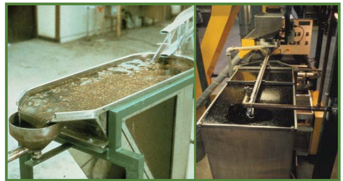
Figure 51 Two different pieces of equipment used for liquid separation.
