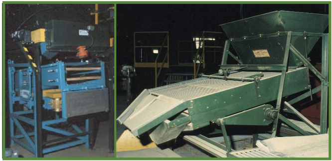
Figure 44 Two types of equipment used to remove released seeds and debris from cones, before kilning.
