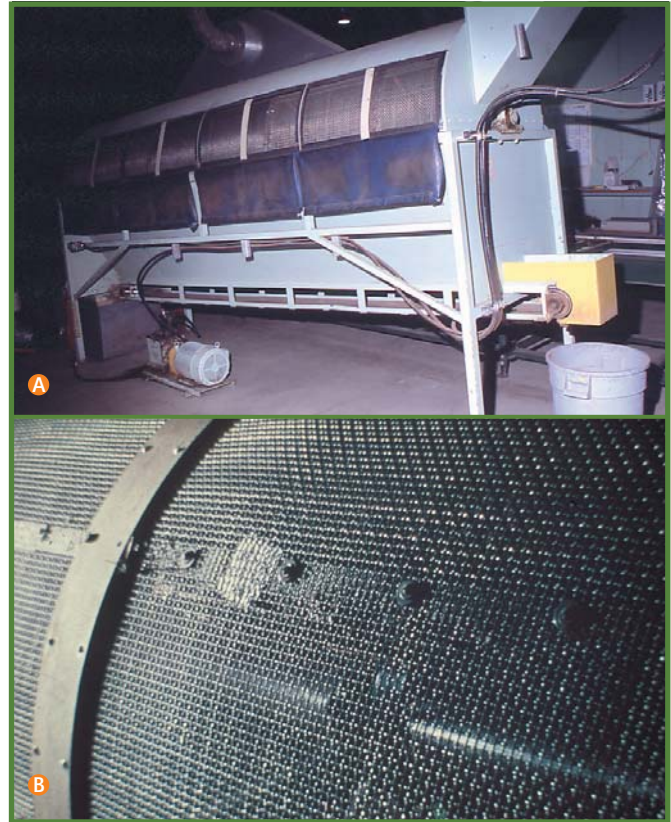
Figure 47 a) A cone tumbler and b) a close-up of the wire mesh screen used to separate seeds from cones.
