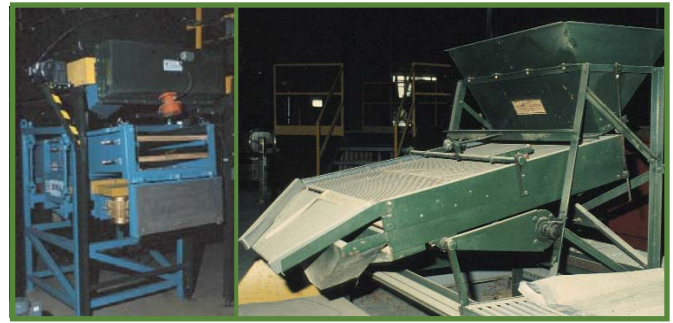
Figure 44 Two types of equipment used to remove released seeds and debris from cones, before kilning.
