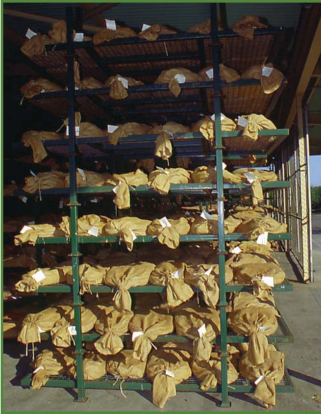
Figure 40 A typical cone sack racking system.
