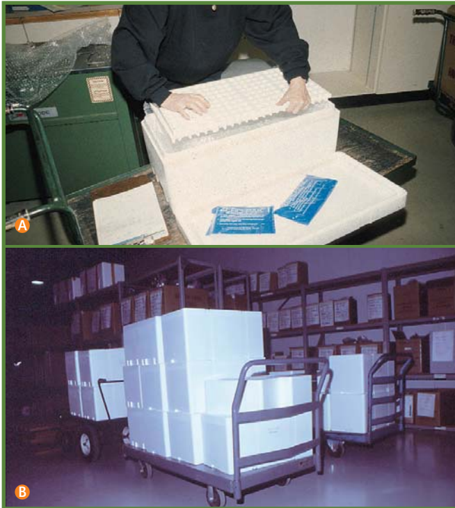
Figure 73 Contents of a seed shipment a) including ice packs and insulating material and b) a seed shipment awaiting pickup in the cooler.
