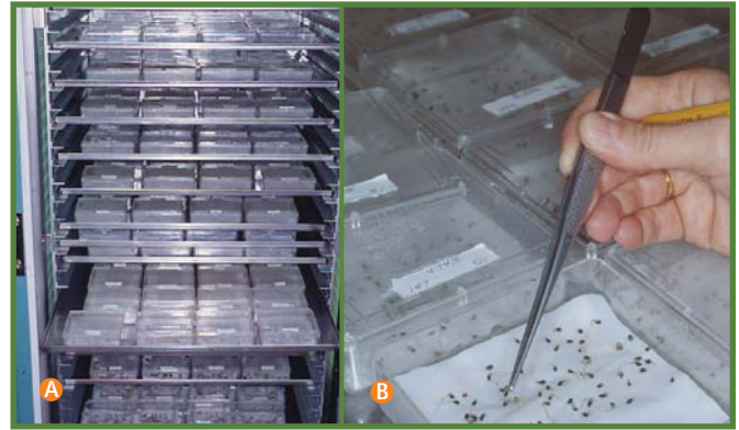
Figure 58 Germination testing a) environmentally controlled germinator and b) counting and removing germinants from dishes.
