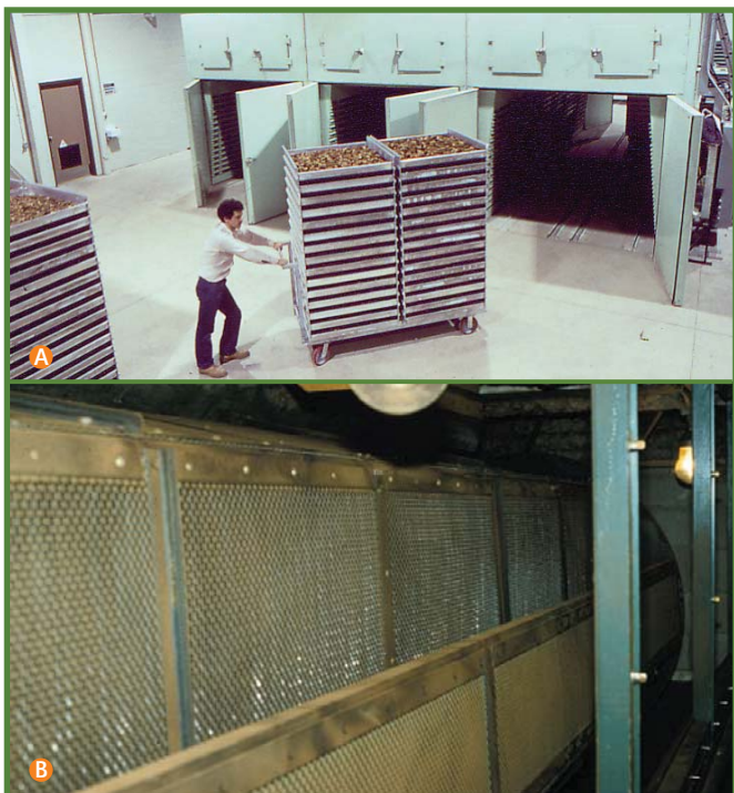
Figure 45 The two main types of kilns used for opening cones a) batch-type and b) rotary.
