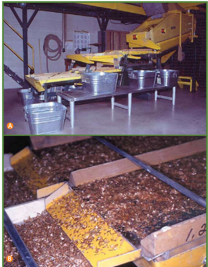
Figure 48 a) Initial cleaning performed on the scalper and b) a close-up of the seeds running over the screens.
