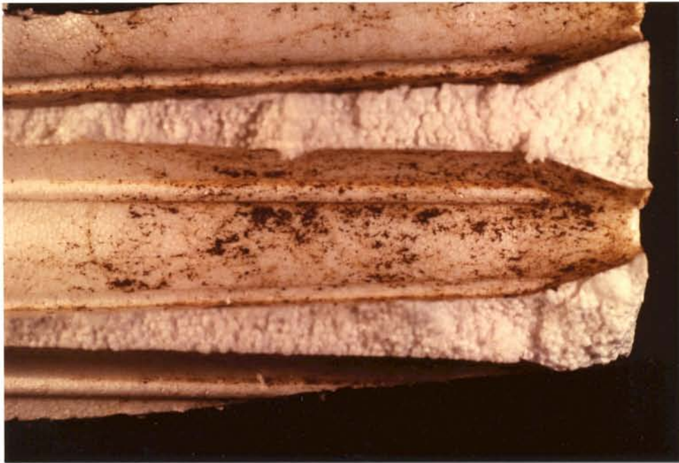
Figure 1. Cross section of a "cleaned" styroblock cell from the Western Forest Systems Nursery. Note abundance of soil mix and other organic material along the inner surface of the cell.
