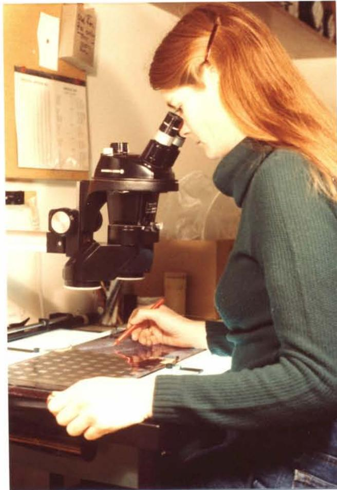
Figure 4.--Bausch and Lomb zoom stereoscope used for photo interpretation.
