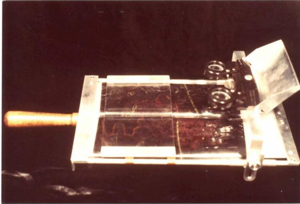
Figure 6.--Photo field viewer used in conjunction with the Abrams CB-1 stereoscope for field delineation of 0.4 ha cells to be surveyed for incidence of root disease damage.
