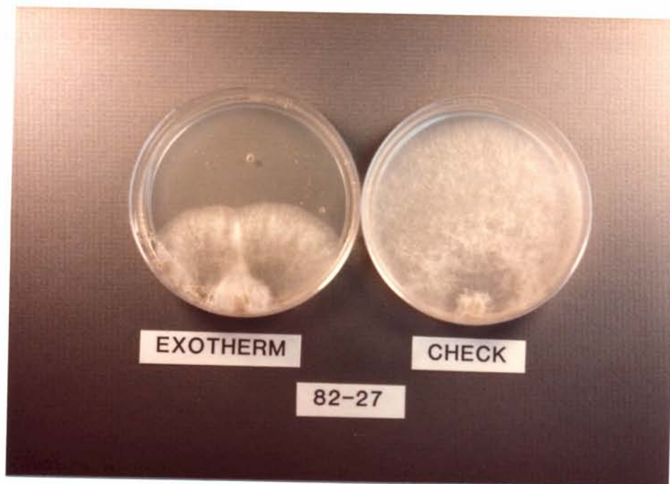
Figure 3.--Growth of Botrytis cinerea (isolate 82-27) on PDA amended with 50 ppm chlorothalonil (Exotherm®) after 6 days. Colonies were fast growing, uniform with abundant aerial mycelium.
