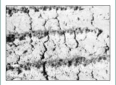
FIGURE 3.1 Heavy clay soils crack and become hard as they dry.
