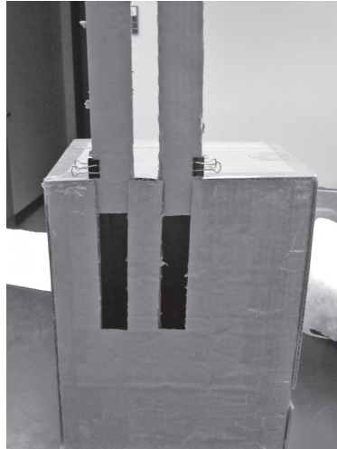
Figure 13. View of the vacuum control gates on the box aspirator.
