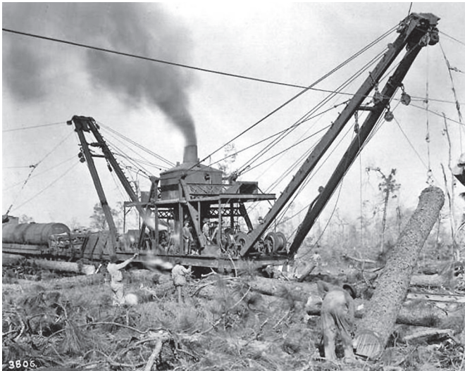
Figure 1. Steam-powered skidders manufactured by the Clyde Ironworks in Duluth, Minnesota, greatly increased logging capability in the early 1900s. Forty acres of timber could be skidded to the railroad track for loading on train cars with one setting of the skidder.
