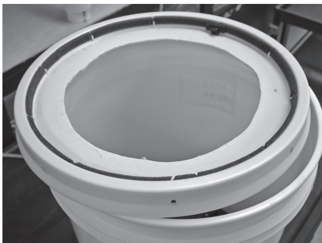
Figure 3. Collar for sealing bucket sized paint strainers when stacked on the pressurized dryer.
