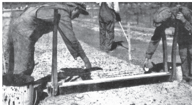
Figure 5. This seed drill for longleaf pine seeds was developed by F.O. (Red) Bateman of the Great Southern Lumber Company.
