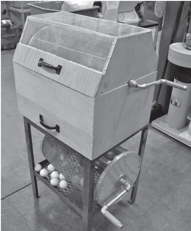
Figure 6. A small hand operated tumbler for extracting seeds from dried open fruits or cones.
