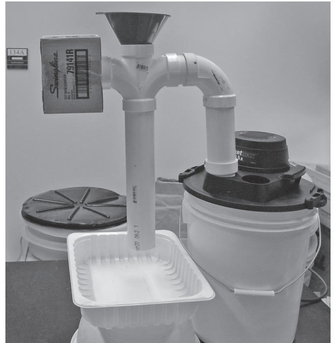
Figure 7. A pipe aspirator made from a shop vacuum and 2 inch (5.1 cm) diameter pvc drain pipe.
