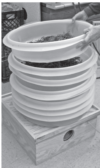
Figure 1. Pressurized seed dryer using barrel sized paint strainer.
