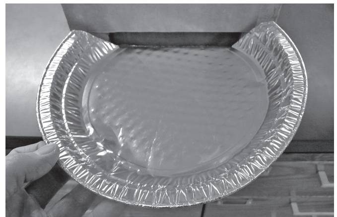
Figure 16. Aluminum pie pan cut to form a hand held feeder to place seeds into the seed chute of the box aspirator.
