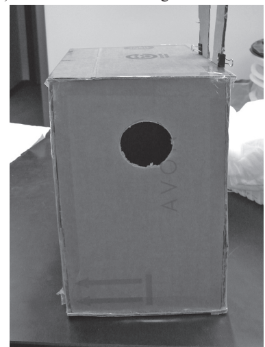
Figure 12. Vacuum source connection for 2 inch (5.1 cm) pipe on the box aspirator.
