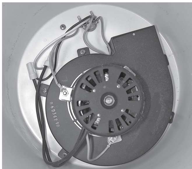
Figure 4. Induced draft blower installed in the pressurized seed dryer.
