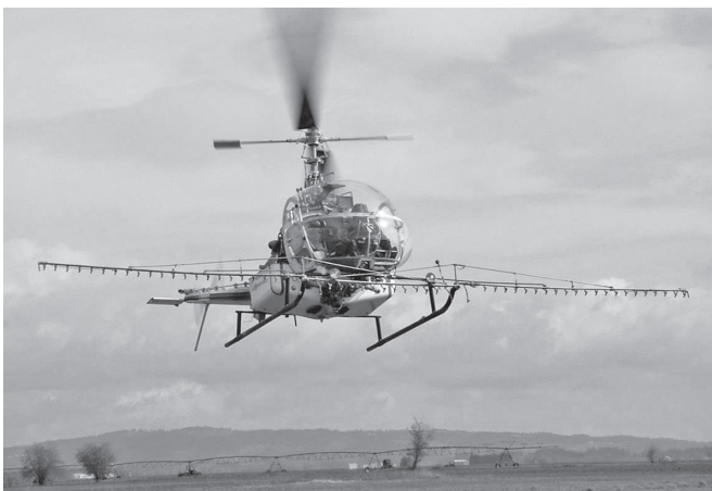
Figure 5. Aerial spraying provides excellent, low cost control of cone and seed insects.
