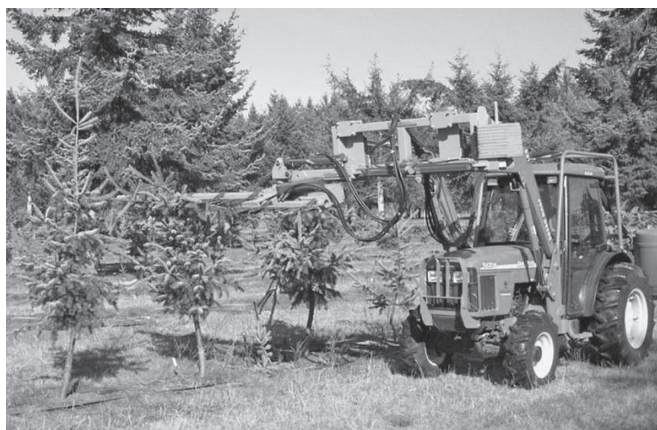
Figure 8. Sickle bar mower for automated tree topping in a Douglas-fir seed orchard.
