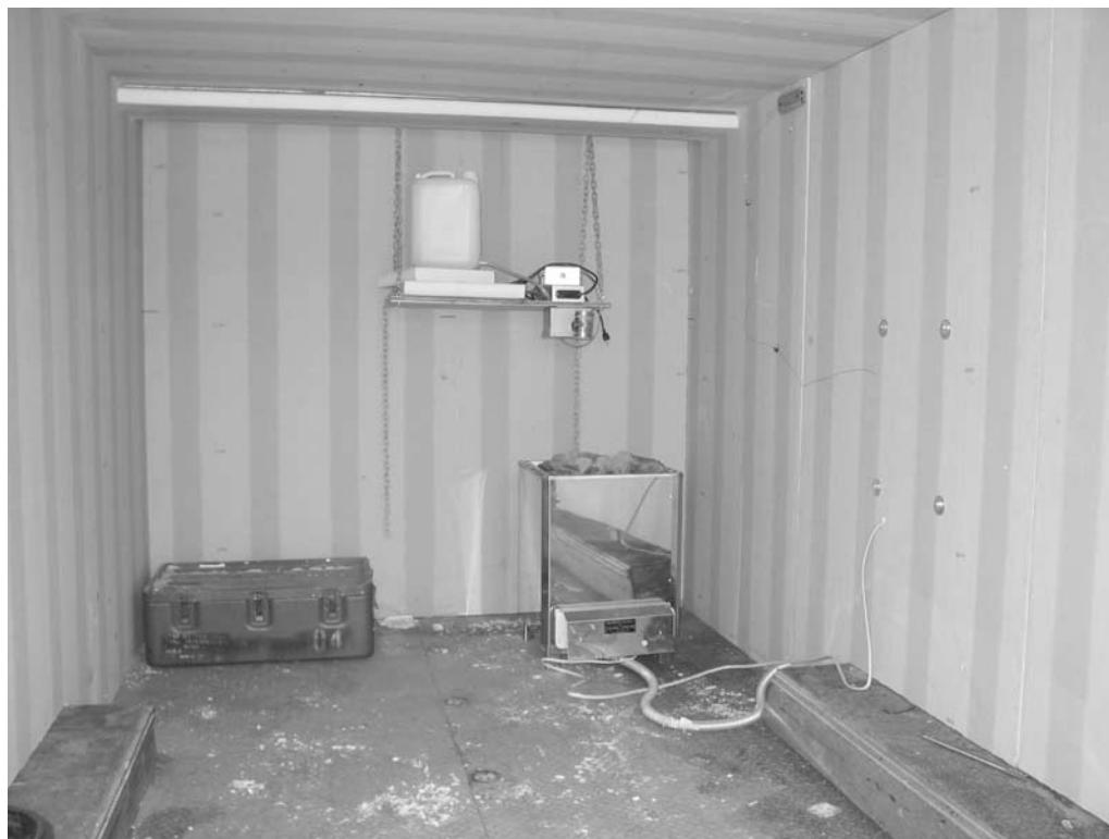
Figure 5 —A storage container outfitted with a commercial sauna heater was used to sterilize blocks during testing.
