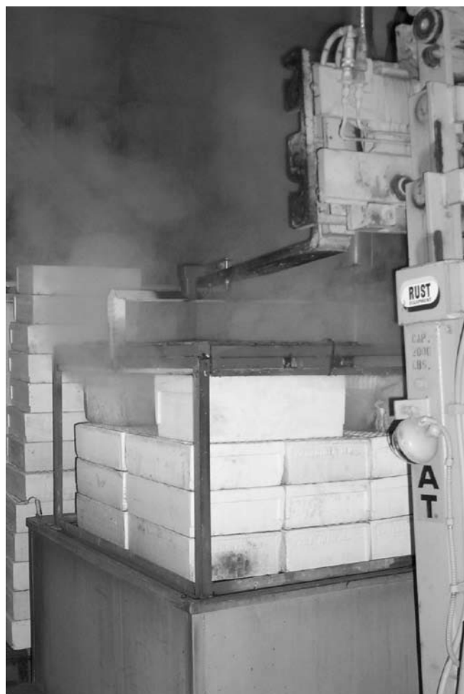
Figure 2 —Blocks are loaded in a cage and submerged in hot water for 2 minutes during the conventional methods of sterilization. A forklift forces the blocks down into the water.
