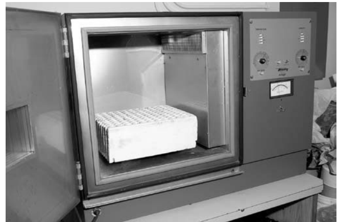
Figure 3 —Blocks were baked in an industrial oven set to 170 °F (77 °C) to determine whether dry heat would sterilize them.
