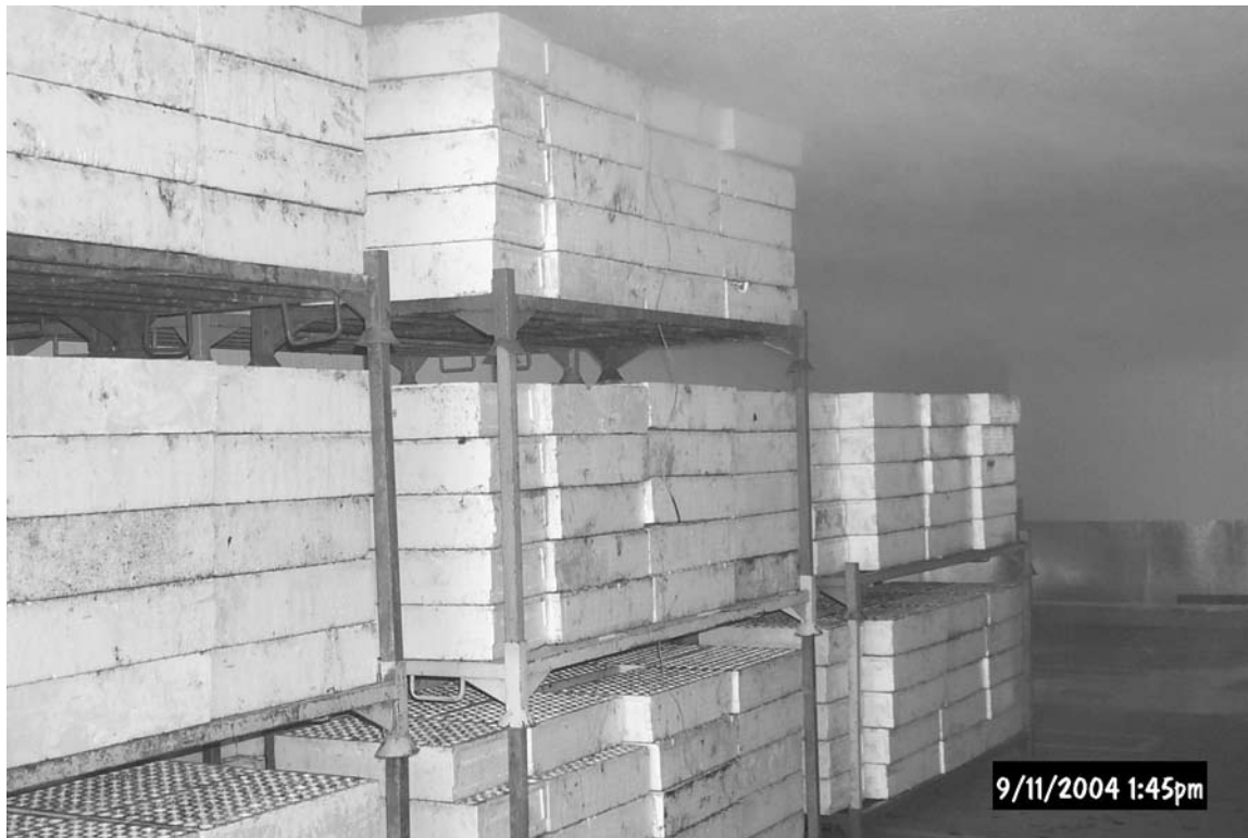
Figure 8 —Blocks are loaded on storage racks inside the sterilization room.
