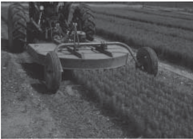
Figure 4 —Rotary mower used to manage seedling shoot growth in bareroot seedling beds.
