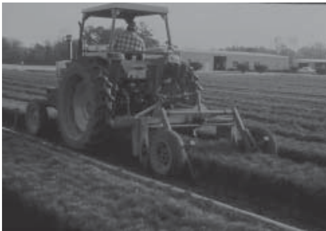
Figure 2 —Reciprocating blade used to undercut root systems in bareroot seedling beds.
