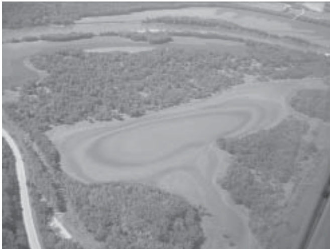
Figure 4 —Approximately 90% of the volume in the 54 backwater lakes along the Illinois River has been lost to sedimentation.
