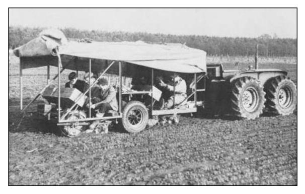
Figure 8. By the 1960s, full-bed transplanting machines could plant 6 to 8 rows at one time. These units were the progenitors of modern transplanters (modified from Aldhous 1975).
