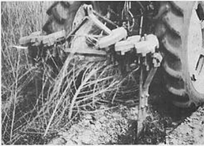
Figure 5. -- Close-up of blade undercutting roots of black willow ( Salix goodingii ) in bare root production.
