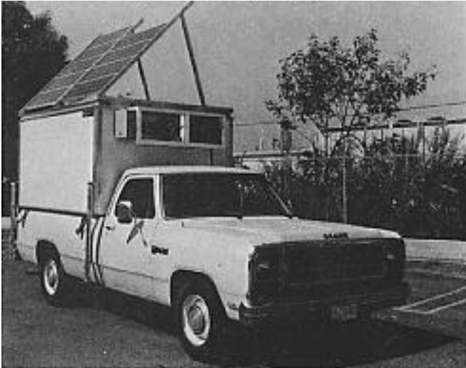
Field Storage Refrigeration Unit
