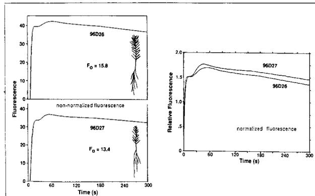
Figure 3.--The normalization operation largely compensates for differences in amplitude of individual White spruce seedling Fv curves. Non-normalized F<sub>0</sub> curves (left) of seedling 961326 and 961327 are from the same seedlot (8981). Their normalized Fv transients are compared in the right.
