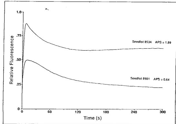
Figure 6.-- Provenance differences in the photosynthetic inactivation of White spruce seedlings. Other data as in Fig. 5.
