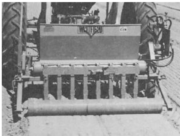
Figure 8.--A commercially available machine applies bands of commercial Pt vegetative inoculum to a bare-root nursery seedbed.
