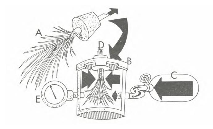
Figure 1 Measuring PMS with a pressure chamber. A, sample; B, pressure chamber; C, pressure tank; D, water forced back to cut surface; and E, pressure gauge.
