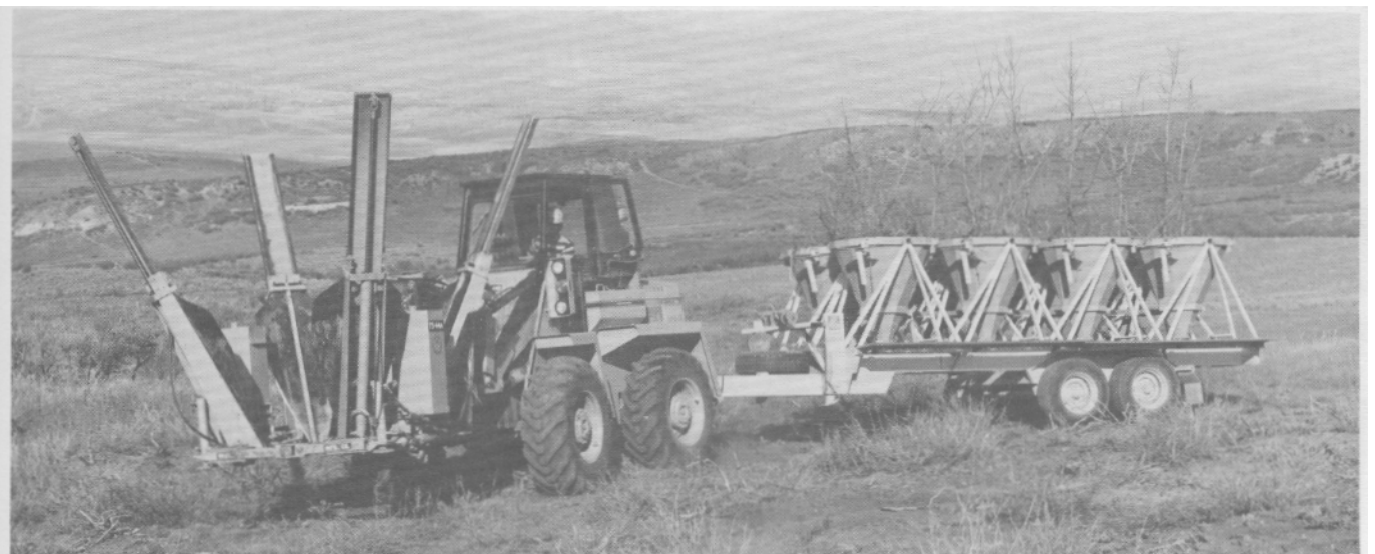
Figure 2.--Tree transplanter revegetates reclaimed mine site with trees and shrubs.
