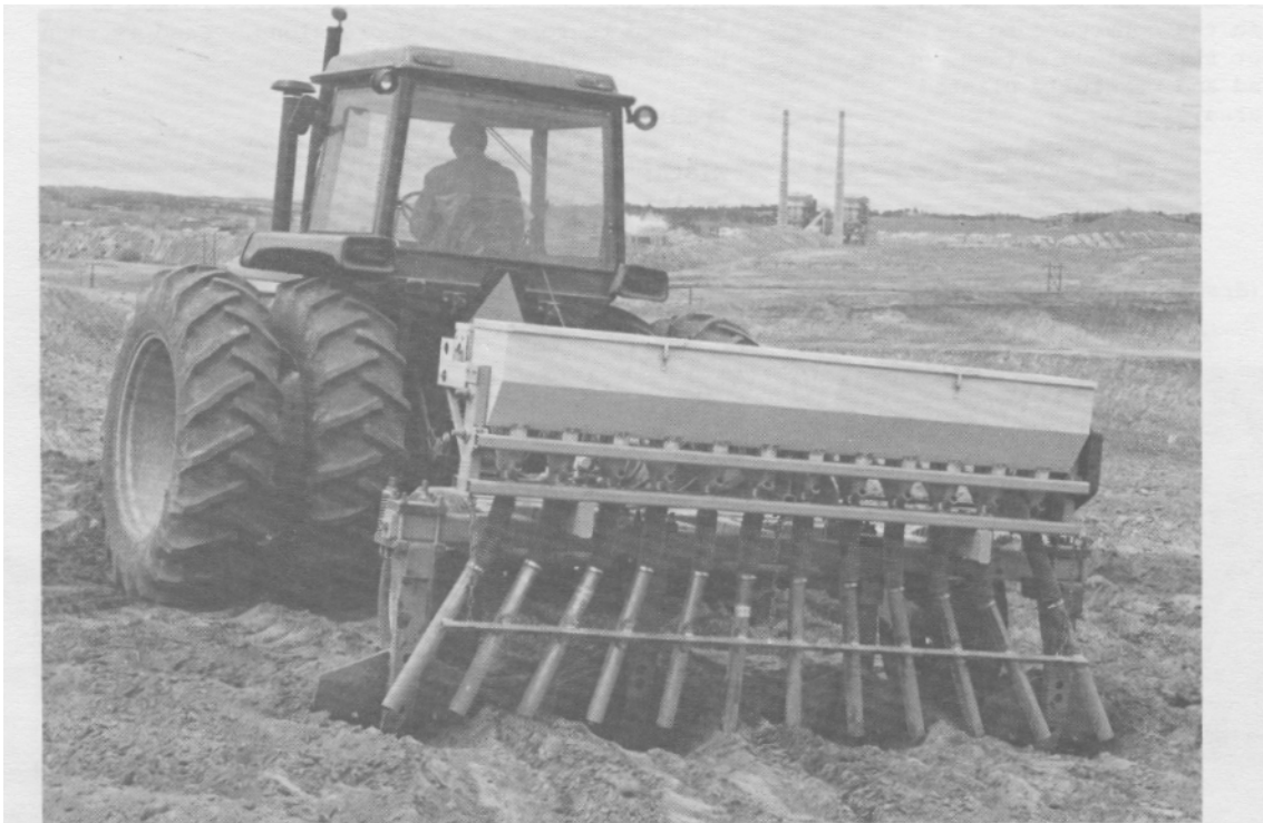
Figure 6.--Hodder gouger makes depressions in soil and simultaneously seeds area to establish plant cover.
