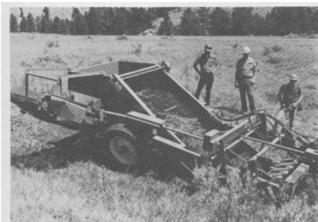
Figure 4.--Sprigger digs up rhizomatous material for planting on reclaimed areas.
