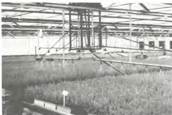
Figure 3. Self-propelled electric irrigation boom watering 12-week-old black spruce.
