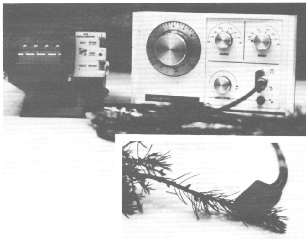
Figure 1. Oscilloscope/square-wave apparatus. Insert: electrode from oscilloscope/square-wave apparatus in seedling terminal.
