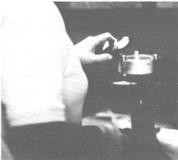
Figure 6. Hydraulic press used to measure moisture stress.
