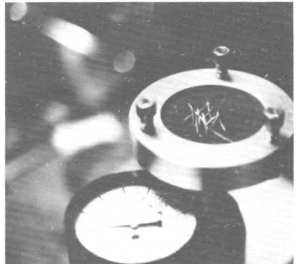
Figure 6. Hydraulic press used to measure moisture stress.
