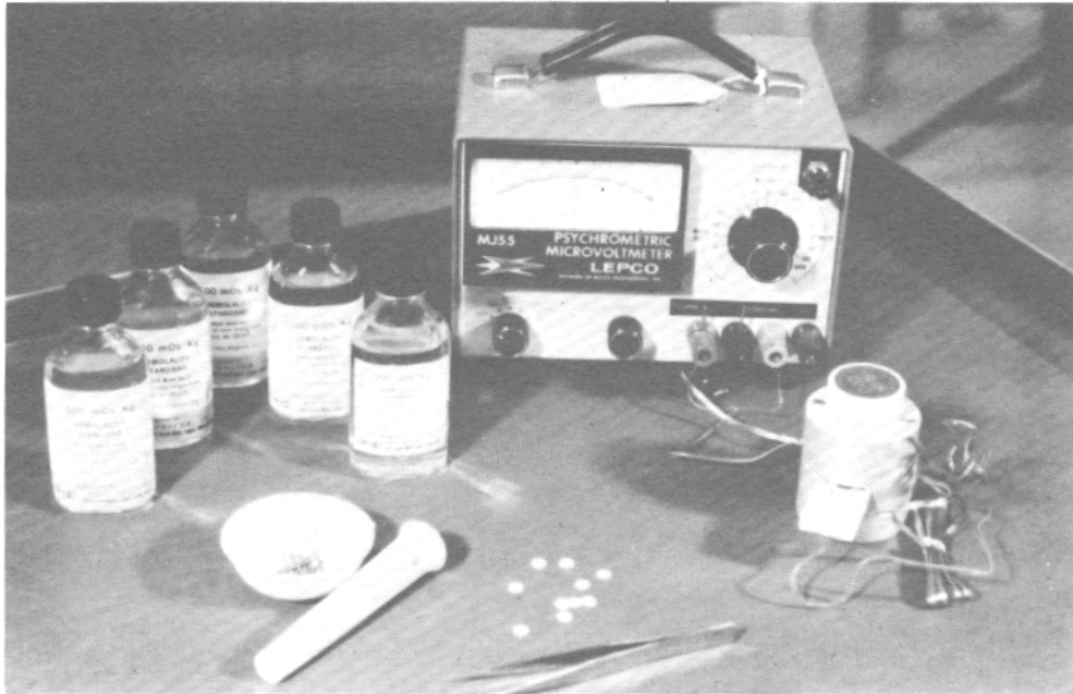
Figure 4. Equipment needed for water-potential studies. Psychrometer chamber apparatus is connected to a microvoltmeter. A paper disc, saturated in tissue water extracted by maceration is inserted in the psychrometer chamber. The equipment is calibrated by known standards.
